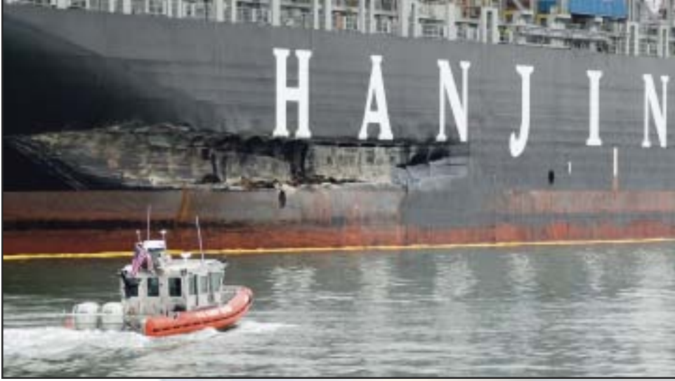
Damage to the 900-foot container ship after its allision with the San Francisco Bay Bridge. USCG photo.
