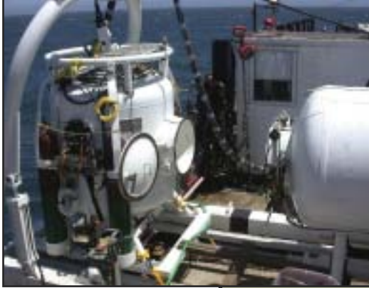
The saturation system used during the SS Jacob Luckenbach response. Photo courtesy of Global Diving and Salvage.
