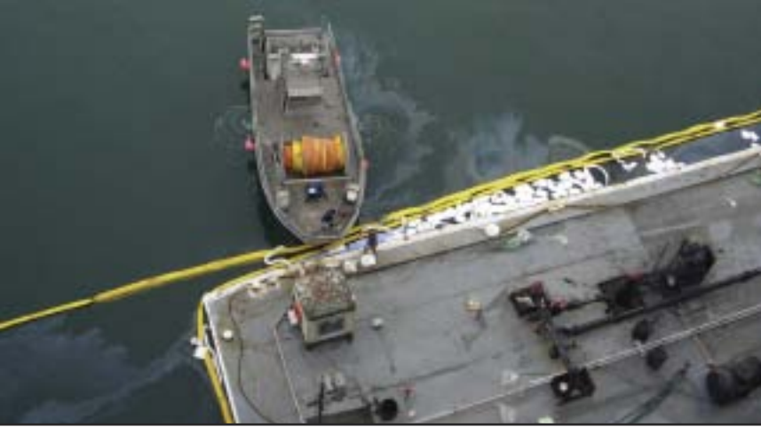
Example of the potentially excessive use of pads during a response to a hydraulic leak from a booming vessel during cruise ship bunkering operations. USCG photo by MK1 Joe Poma.
