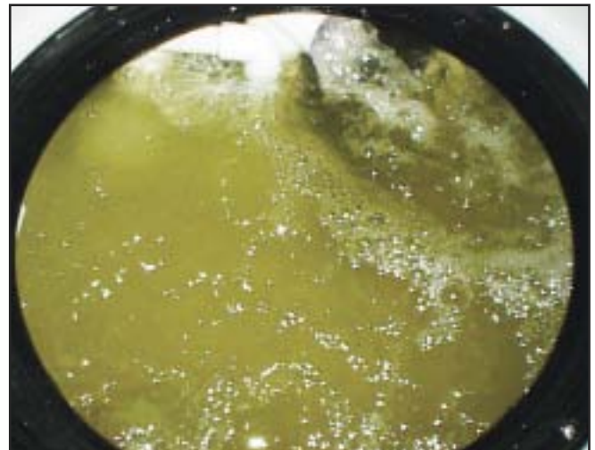
Aerobic digestion of sewage waste by biological device. Courtesy TEi-Testing Services.
