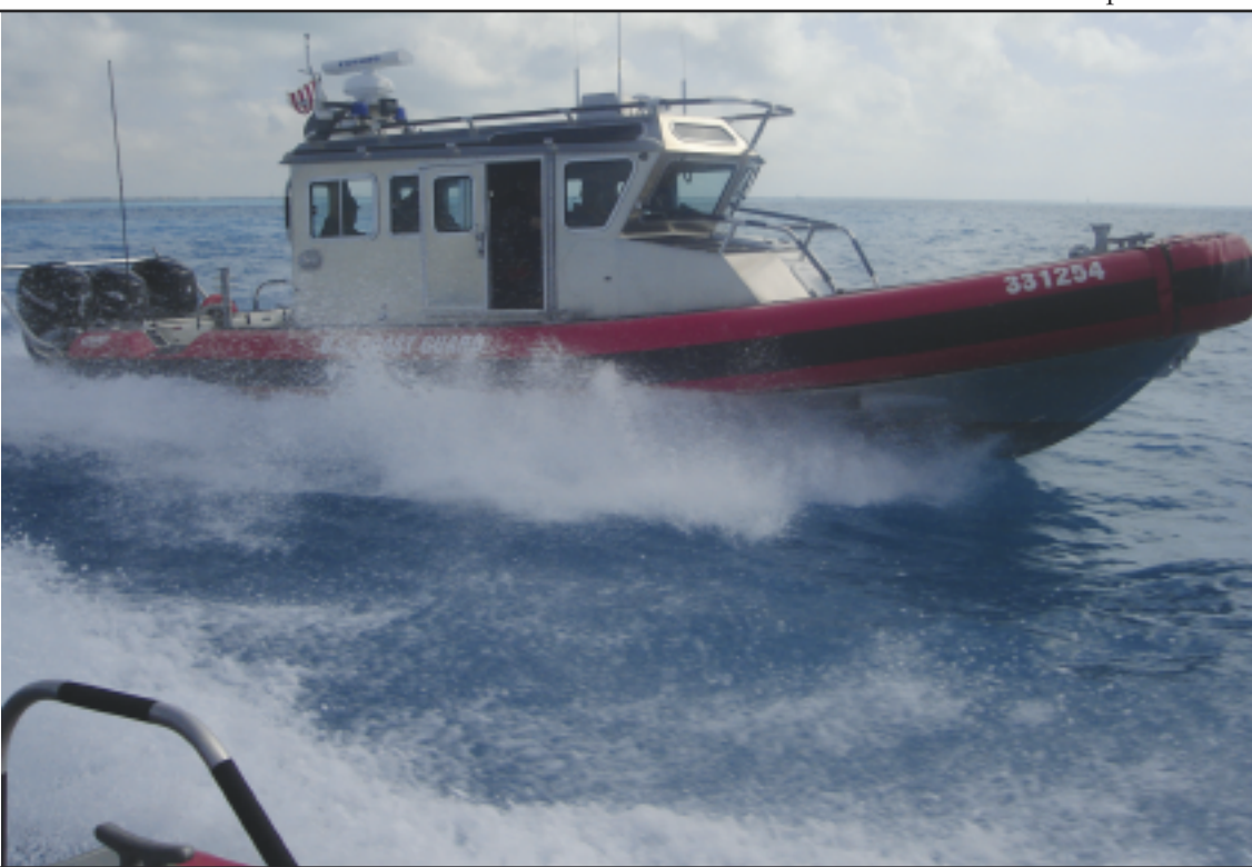
The new special purpose craft—law enforcement boats have a top speed of over 50 knots and are intended to enhance offshore capabilities of Boat Forces units. USCG photo.
