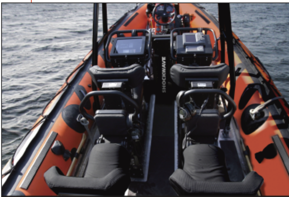
Shock-mitigation seating arrangement for crewmembers onboard a CB-OTH MKIII. Note the electronics “ride” in the same pods as the navigator and communicator positions. Photo courtesy of Shockwave Marine Inc.
