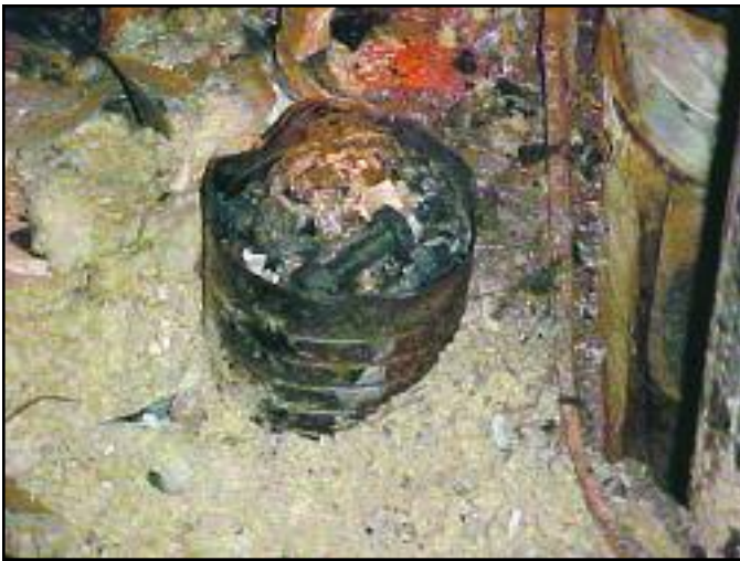
Fire damage to equipment and gear on the 03 level of the engine room. USCG Photo.
