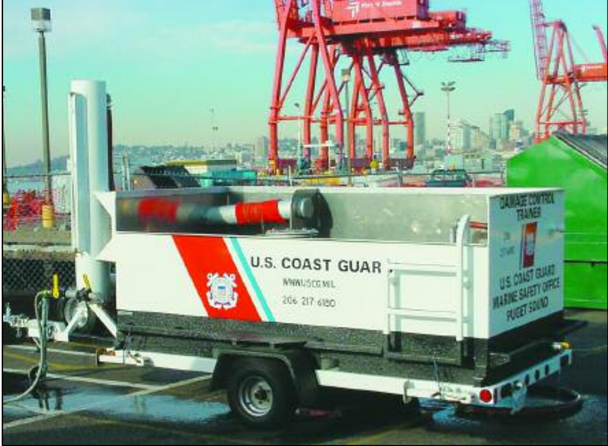
Figure 1: Damage control trainers are used to illustrate damage control procedures and increase awareness of typical flooding risks.
