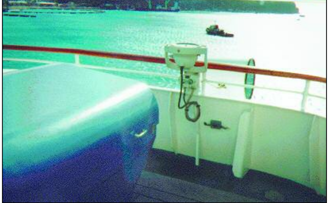
Figure 3: The exterior starboard bridging repeater. USCG photo.
