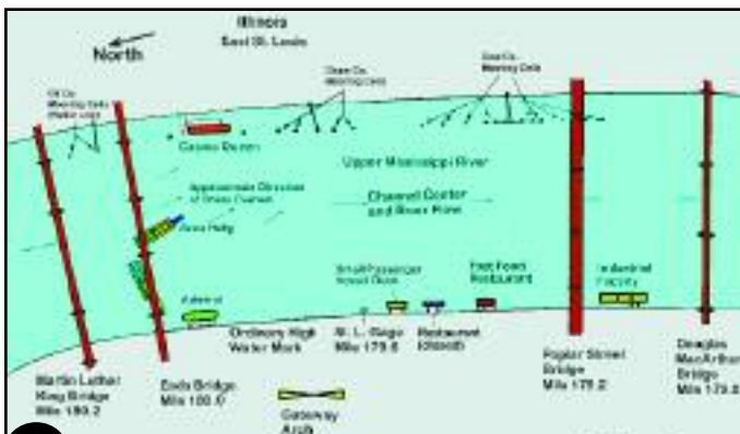
4 Partway under the bridge the vessel stalls, and the current causes the tow to drift sideways, pushing barges into a bridge support and breaking the tow coupling.
