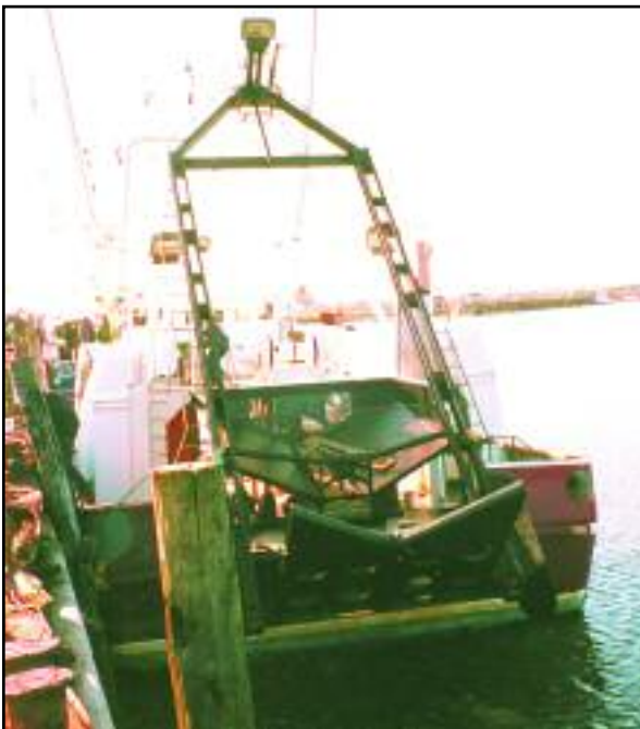
Stern of Beth Dee Bob after refit showing the "A" frame and dredge. The two new "dog houses" are visible on either side and in front of the dredge. USCG photo.
