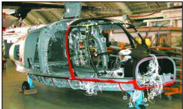
Figure 5: The Deepwater Program's re-engining of HH-65 helicopters has been accelerated as the Coast Guard's top aviation priority. Three re-engined HH-65C helicopters performed superbly during Hurricane Katrina rescue operations, saving 305 lives during 85 missions. As depicted here, older model helicopters undergo a comprehensive modernization during the re-engining process. PAC Jeff Murphy, USCG.
