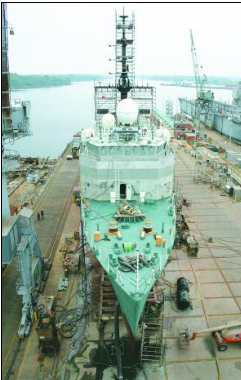
Figure 3: The medium endurance cutter USCGC Tampa sits high and dry at the Coast Guard Yard, Baltimore, Md., during a major systems refurbishment as part of the Mission Effectiveness Project for 210-ft. and 270-ft medium endurance cutters. Gordon I. Peterson, USCG.
