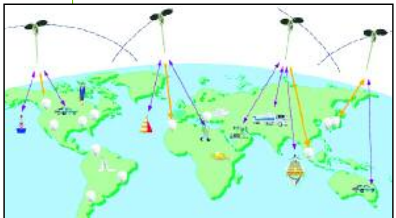
Figure 5: Satellite-based automatic identification system. Courtesy ORBCOMM.
