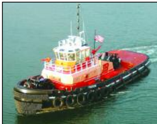
The tug Freedom, a tractor tug, provides port-wide service. Courtesy SUEZ LNG NA and DISTRIGAS of Massachusetts.
