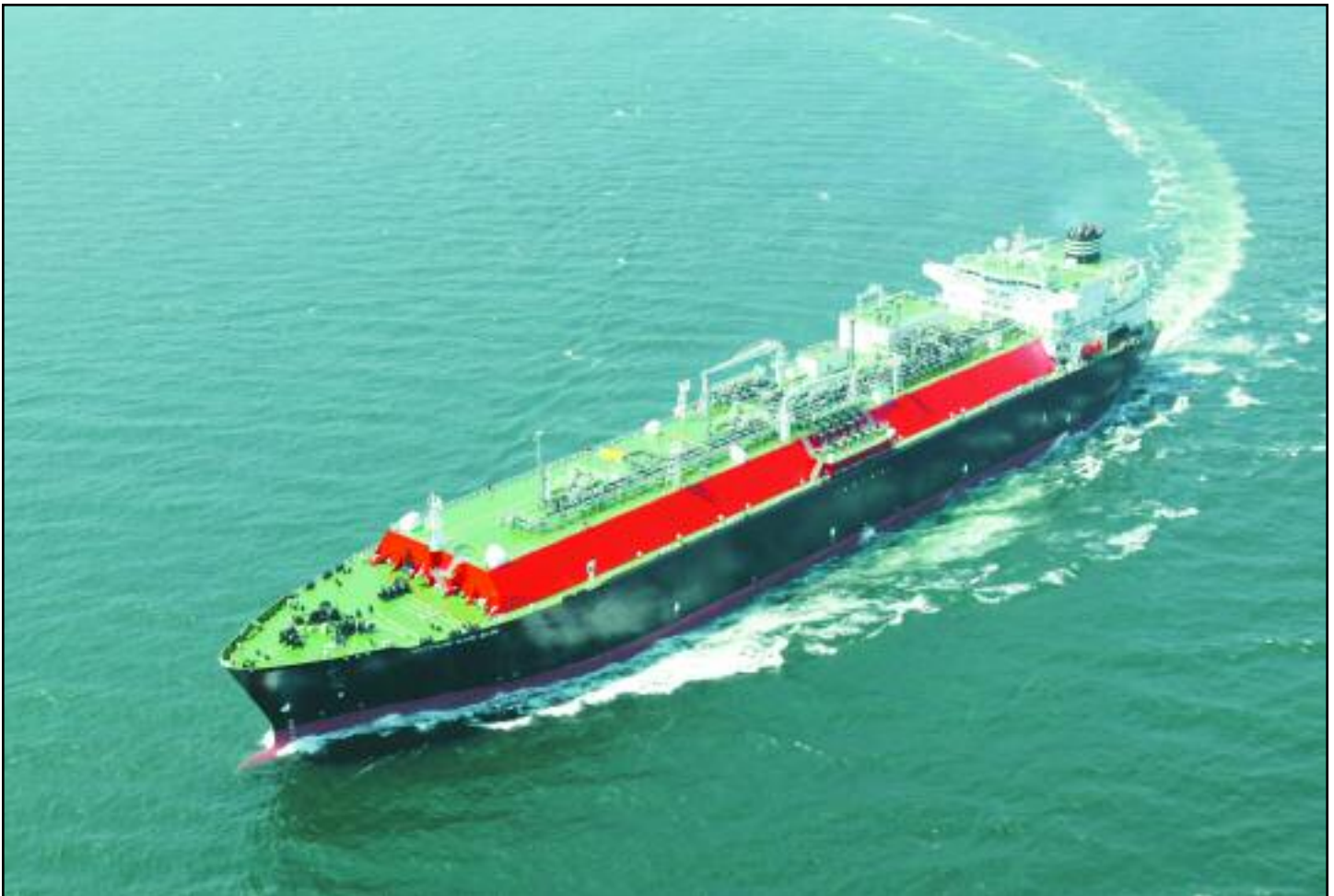
Figure 1: The Methane Kari Elin is BG's newest LNG carrier. The vessel has a cargo capacity of 138,200 cubic meters, with an overall length of 279 meters, a beam of 43 meters, and gross tonnage of 93,410 tons.
