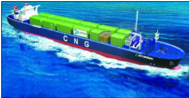
Figure 1: In this ENERSEA design, the ship contains arrays of vertically positioned steel cylinders within insulated holds.
