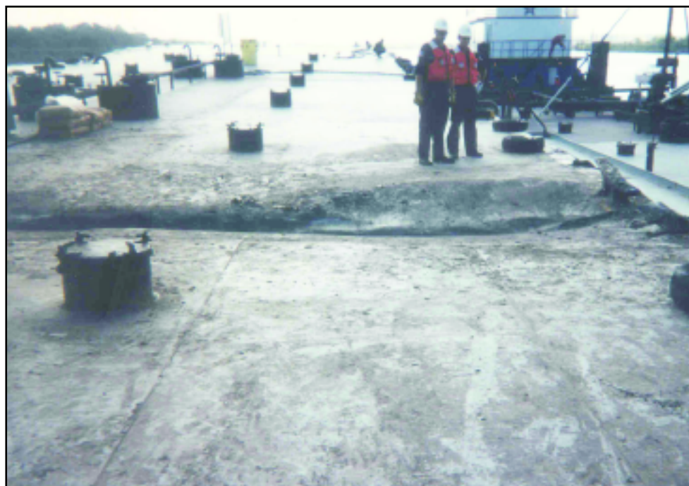
Top: Structural damage at the deck knuckle of Buffalo 292 following compressive failure of the tank top. Bottom: Compressive loads in the Buffalo 292 tank top resulted in global structural failure, evidenced by a sharp crease and several tears along the breadth of the barge. Both courtesy MSU Galveston.
