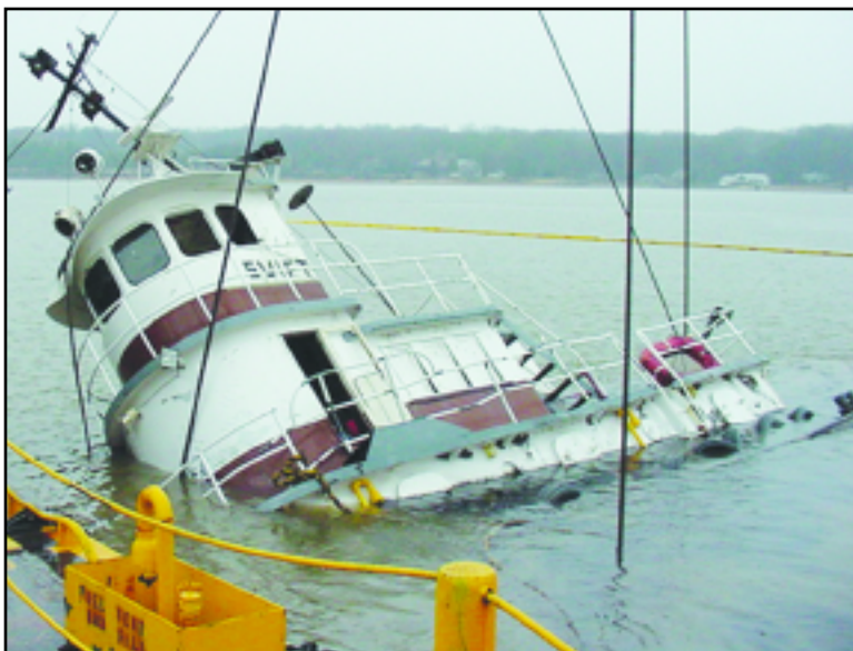
In February 2002, the Swift collided with a bulk cargo vessel. SERT provided on-scene support and approved the salvage plan consisting of lifting, righting and dewatering the vessel. Courtesy SERT.
