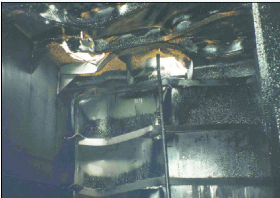
Top: Structural damage at the deck knuckle of Buffalo 292 following compressive failure of the tank top. Bottom: Compressive loads in the Buffalo 292 tank top resulted in global structural failure, evidenced by a sharp crease and several tears along the breadth of the barge. Both courtesy MSU Galveston.
