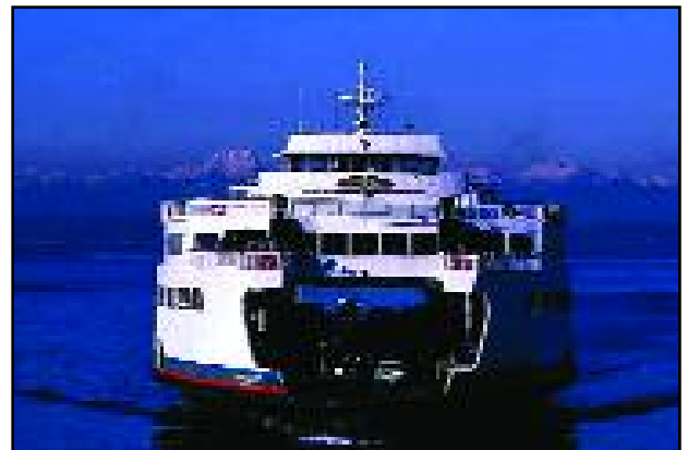
The Washington State Ferry Spokane can carry 2,000 passengers and up to 206 vehicles. Steven J. Brown, courtesy Washington State Ferries.
