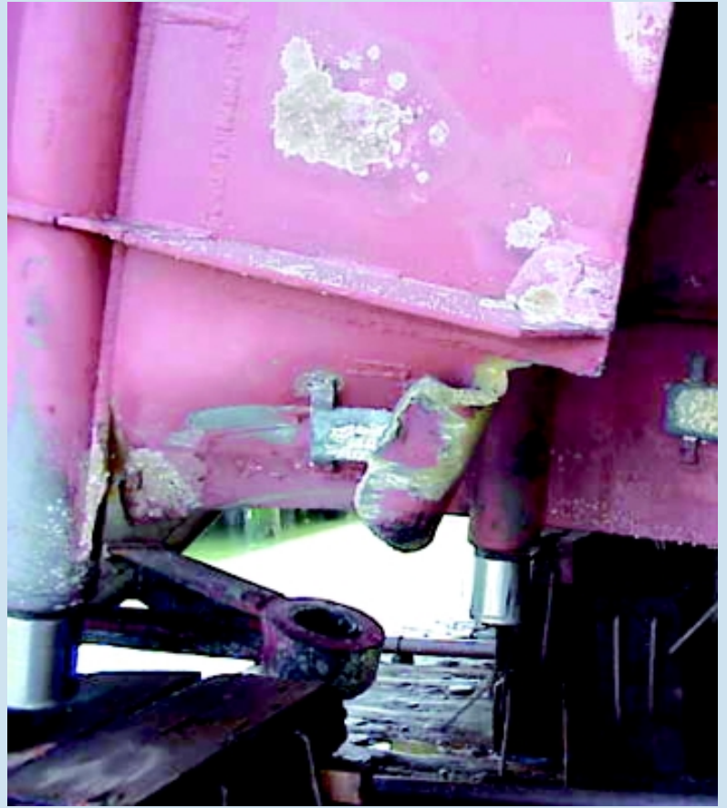
Top: Damage to the lower starboard side; Bottom: The outboard kort nozzle.
