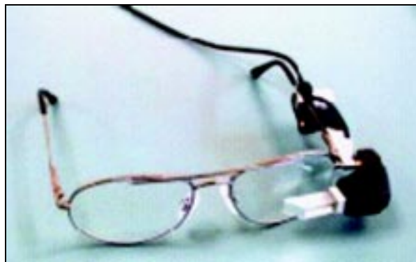
Figure 3. Prototype augmented reality eyewear employing miniature projector.
