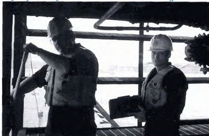
Coast Guard petty officers take current readings with a 20-foot pole and flow meter under the Conrail Bridge.
