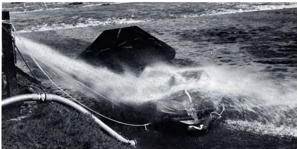
Liferaft canopy closure tests like this usually require the assistance of the local fire department.
