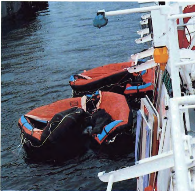
Three of four rafts inflated in about a minute. The fourth took about two minutes to fully inflate.
