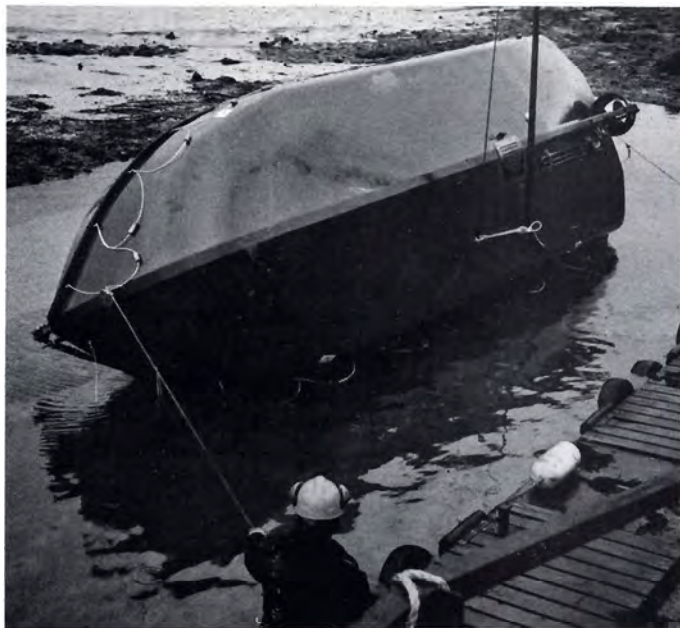
The "righting test" for lifeboat approval is a difficult and expensive proposition.
