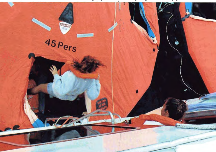
Although ladders were available for boarding, many test volunteers jumped down about four feet to the raft floor.
