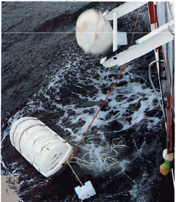
Rafts are deployed. Small floats ease recovery of case halves.
