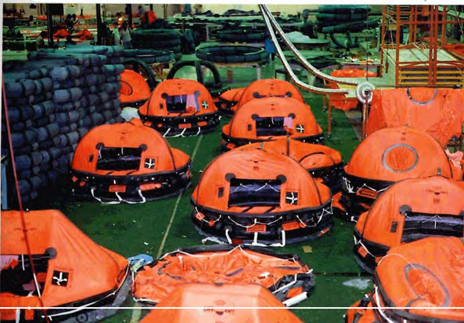
All new inflatable liferafts undergo leakage tests.
