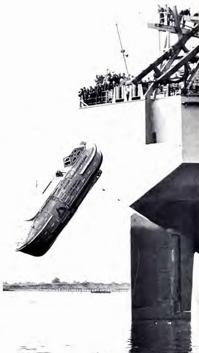
A free-fall lifeboat is launched over the stern of a ship during installation testing.
