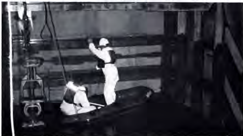
The enhanced survey guidelines require close-up tank surveys such as this.
