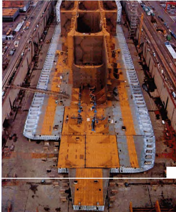
Mobil's double-hull oil carrier, Eagle, is being constructed in Japan.
