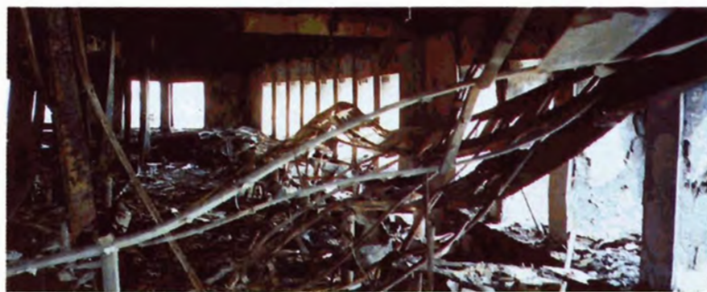
Damages caused by fire on the passenger ship Scandinavian Star in April 1990.
