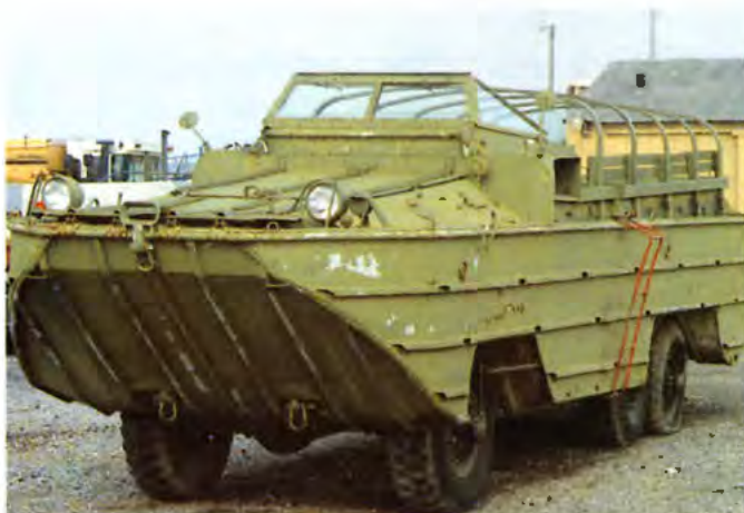
Tires could be deflated for beach landing and re-inflated while moving. Note rust alongside of DUKW.
