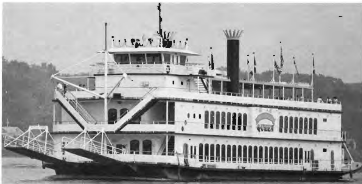
Super T river excursion boat Quad City Queen is 135 feet long and is certified to carry 799 passengers.
