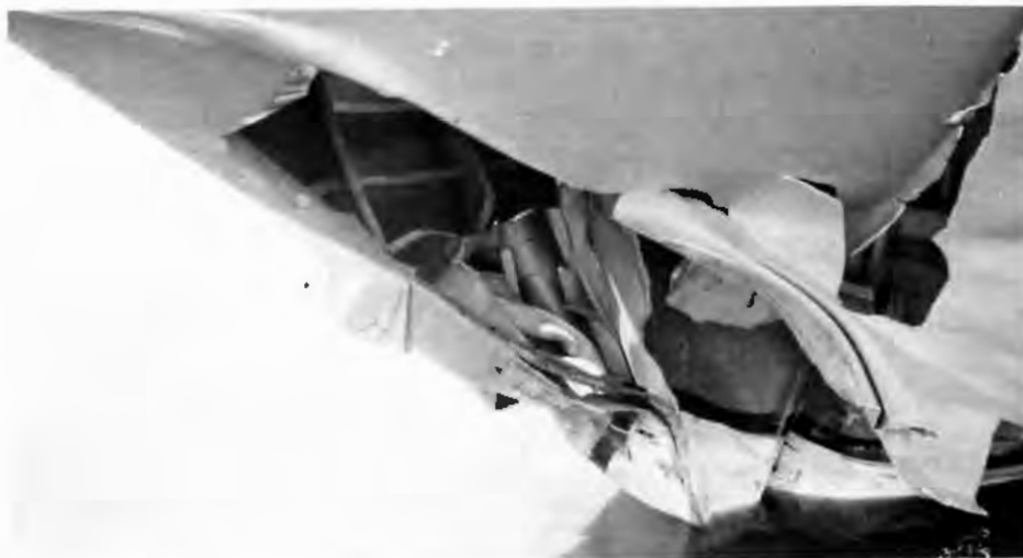
This charter vessel sustained an 8 x 9 foot hole in its bow after colliding with a wellhead in the Gulf of Mexico last year.
