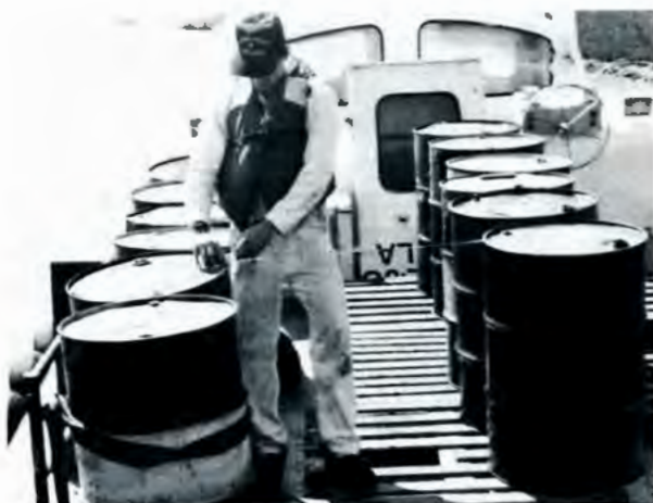
Inspector measures distance test weights have moved across the deck. Total weight times distance must be at least equal to the greater of the passenger or wind heel moments.
