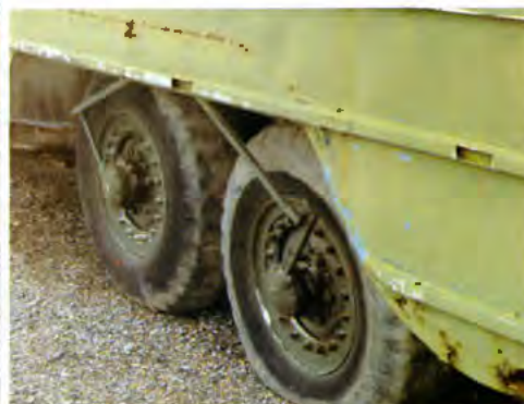
Tires could be deflated for beach landing and re-inflated while moving. Note rust alongside of DUKW.
