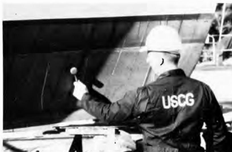
Inspector checks integrity of wood hull during drydocking.
