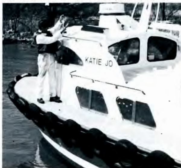
Inspector measures deckhouse height to figure wind area.
