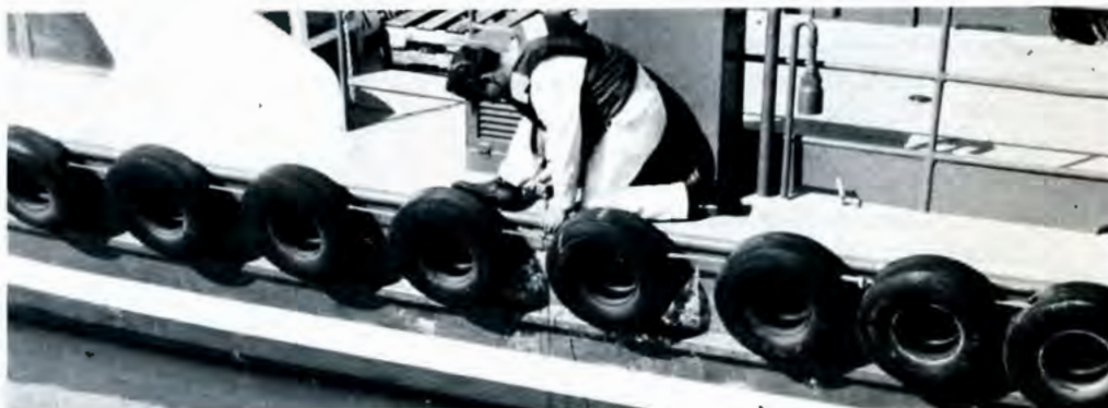
For this flush deck vessel, the maximum immersion mark is placed at one half the freeboard after weights are added.
