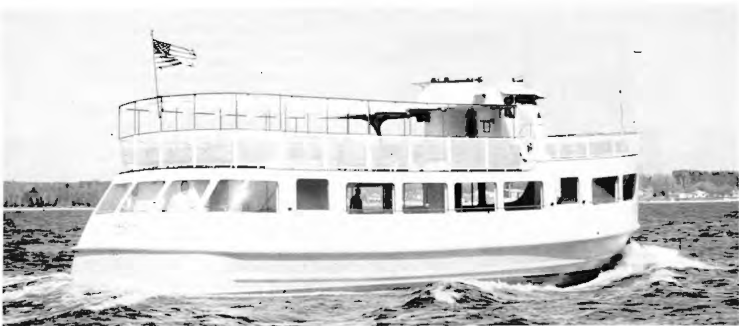
Built in 1961, the 70-foot Marlyn's sloping main deck qualified it as under 65 feet.
