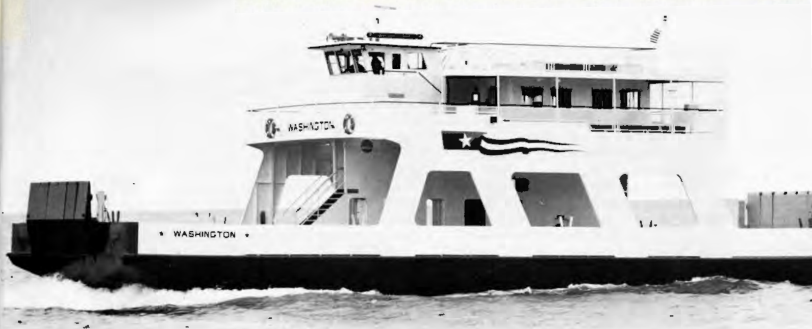
A typical Lake Michigan passenger/vehicle ferry, Washington , can carry 250 passengers, and between 24 and 26 automobiles.
