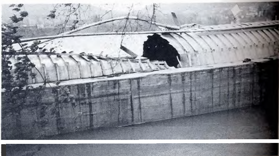
The tank barge DM 973 as it appeared after the explosion collapsed the three transverse bulkheads between the cargo tanks.
