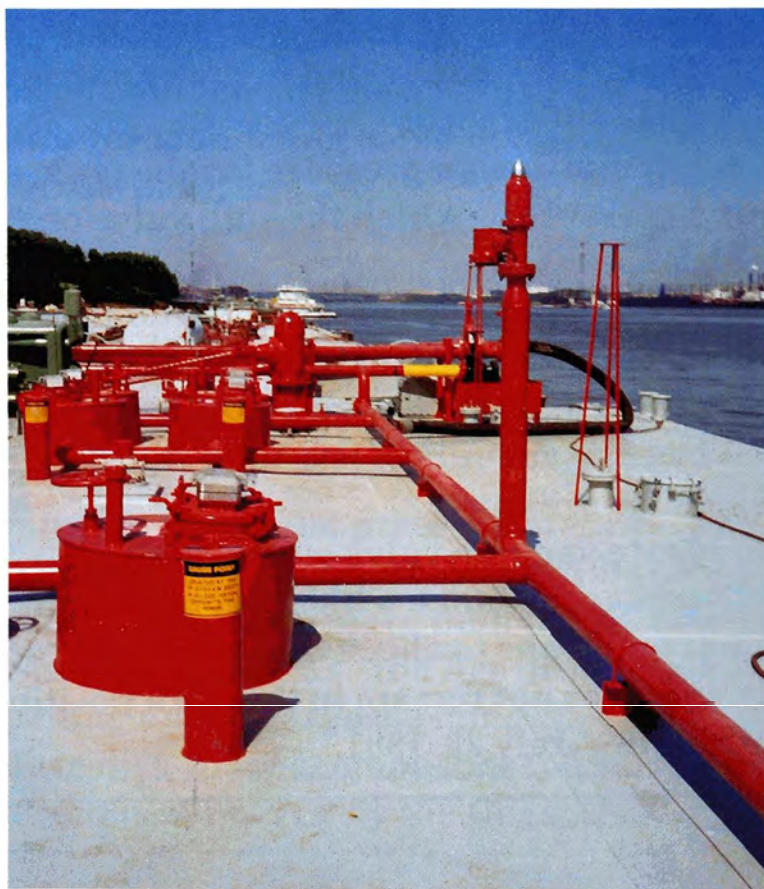
Cargo tank venting system shows "bullet-" type pressure vacuum valve.
