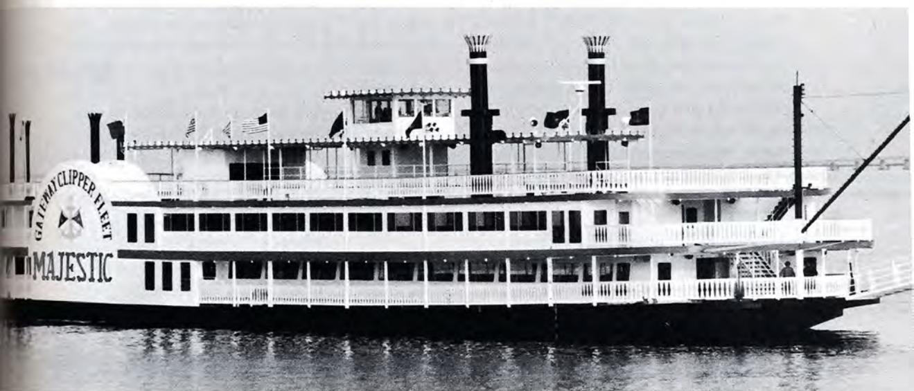
Gateway Clipper Fleet's Majestic has the authentic look of the old steam-powered, paddle wheel ships, but it is actually a towboat and barge configuration. The paddle wheel facade on each side of the vessel hides where the towboat (aft) and barge (forward) actually meet. The captain pilots the passenger ship from the superstructure on the upper deck of the barge.
