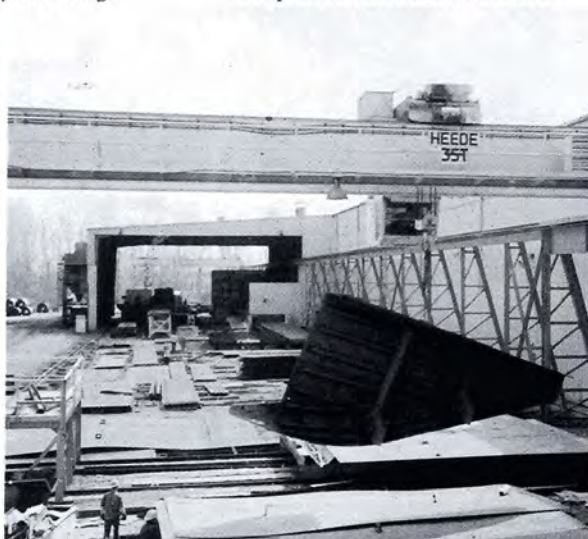
(Left) Wing voids are lifted and fitted into place for welding.
