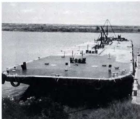
Typical flush-deck type III hull
