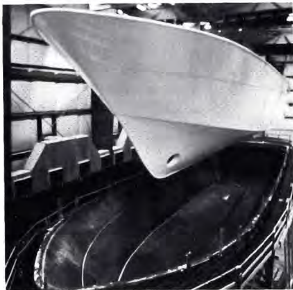
Like popping cakes from a pan . . . A finished hull is removed from a mold
