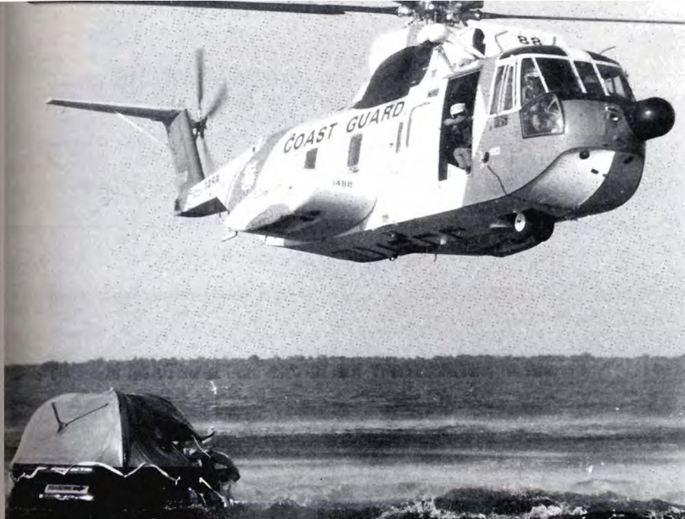
An HH-3 helicopter nears a Coast Guard-approved inflatable life-raft to determine its stability in high winds.
