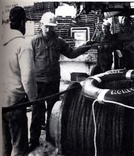
Inspector examines machinery guards on fish reel and the condition of a ringbuoy. Photo by PA2 Don R. Wagner.
