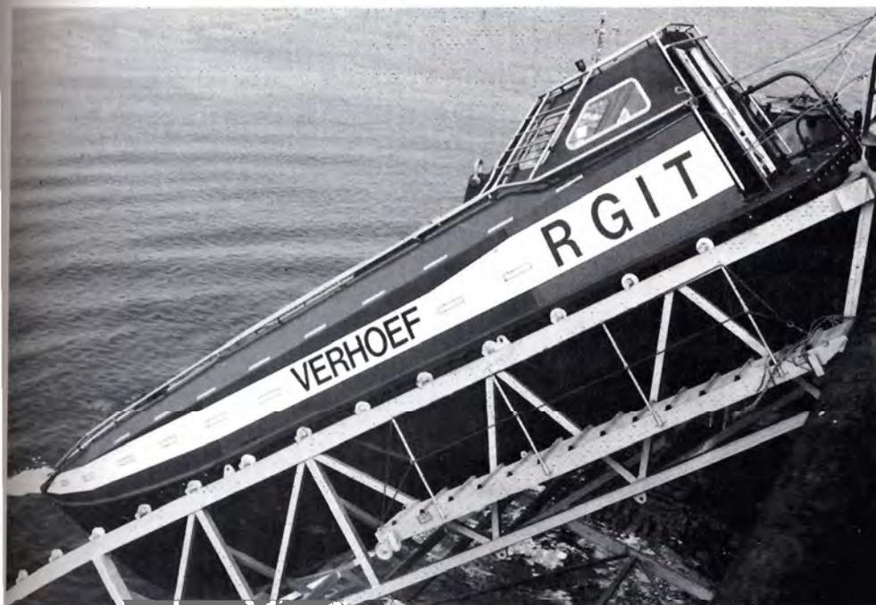
Totally enclosed, fire-protected, aluminum lifeboat is stowed on an inclined ramp in a ready-to-launch position.
