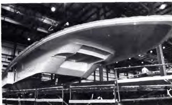
. . . a finished deck is lifted from another mold.
