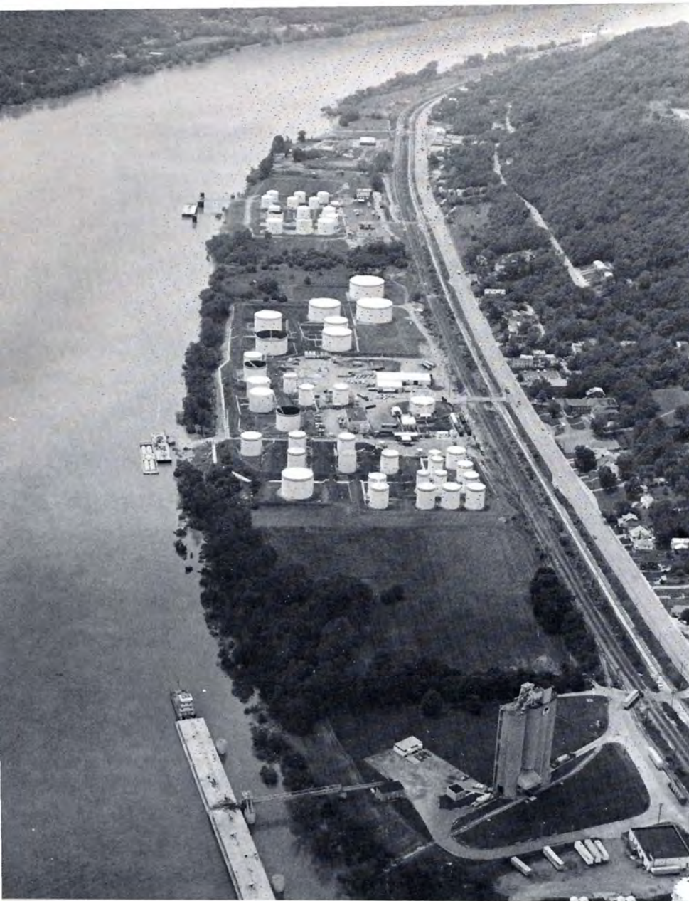
The Ashland Oil Terminal in Cincinnati, Ohio, receives refined petroleum products and chemicals by barge on the Ohio River, and transports them by tank truck and rail car.
