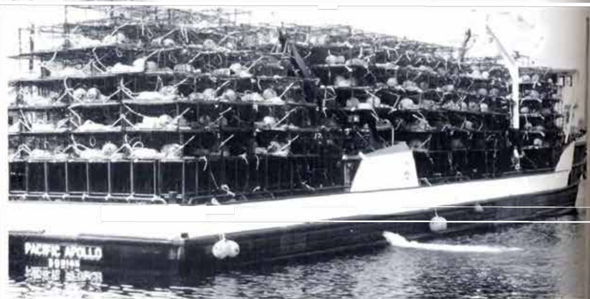
Crab fishing vessels carry high, heavy deck loads. This practice can threaten the vessel's stability.
