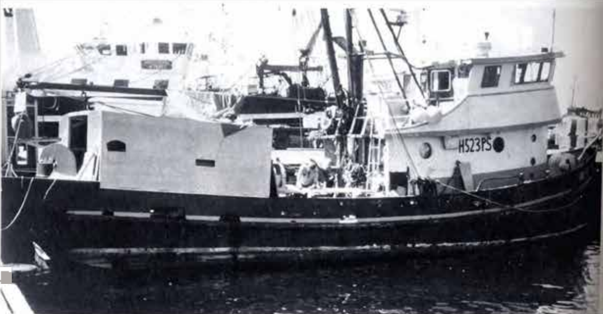
Longline fishing vessels may add shelters on aft decks, increasing the height of the center of gravity.
