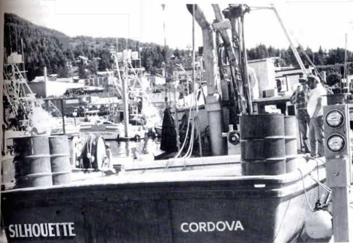
Long pendulums hung in the hold and drums filled with water are used to heel the vessel in an inclining experiment.
