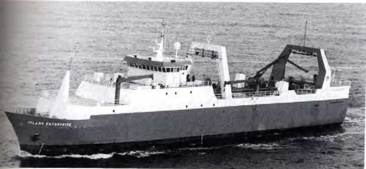
A typical large factory trawler, this vessel can produce up to 80 tons of surimi per day.
