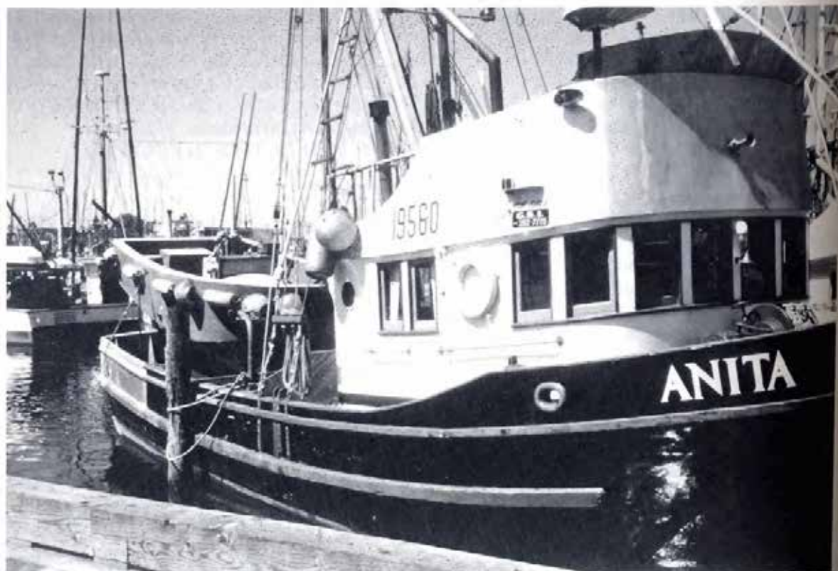
A seine skiff on deck can have an adverse effect on stability
