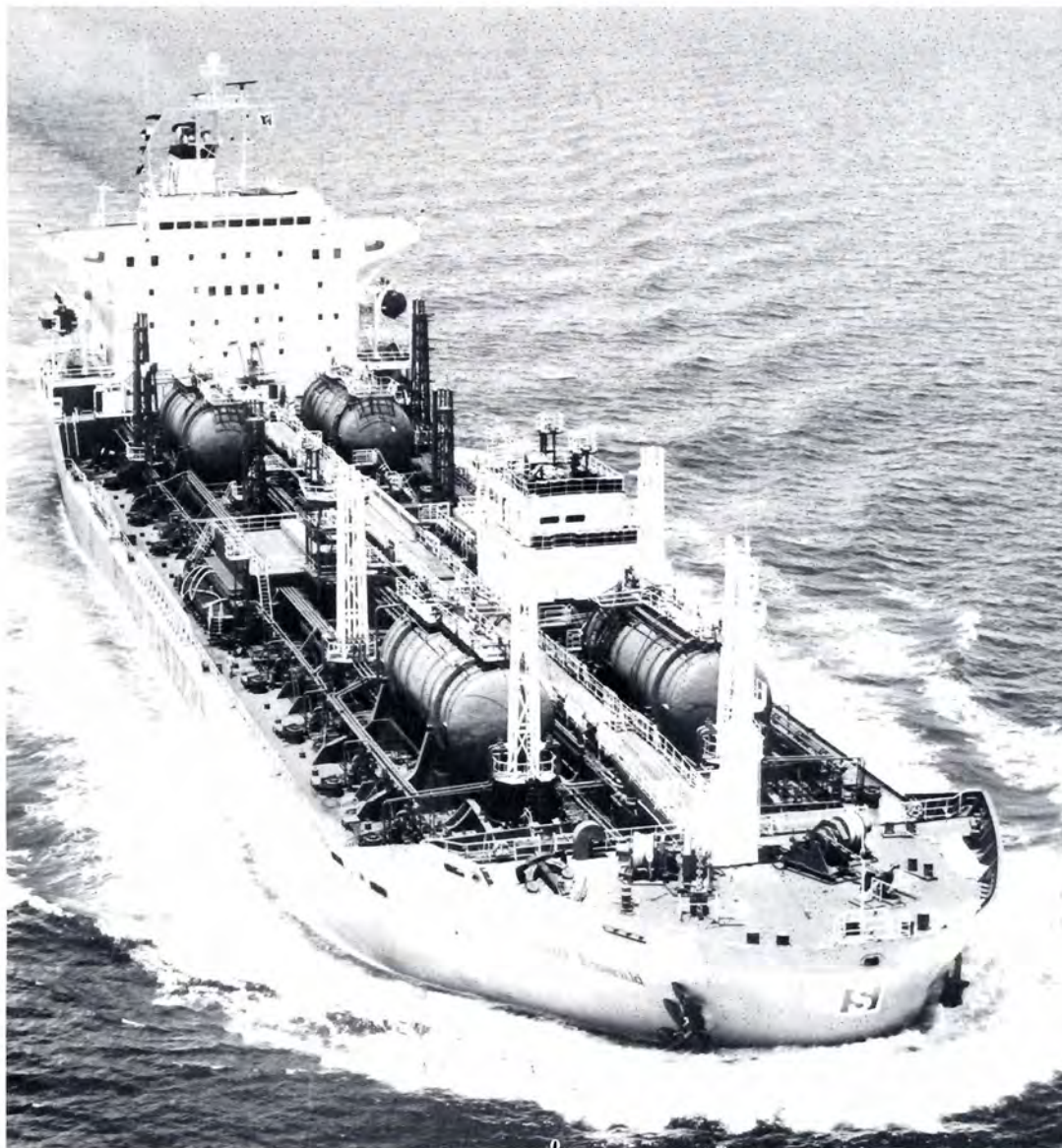
M/T Stolt Emerald , a 38,720-dwt parcel tanker, has 58 segregated tanks. Photo courtesy of Stolt-Nielsen, Inc.
