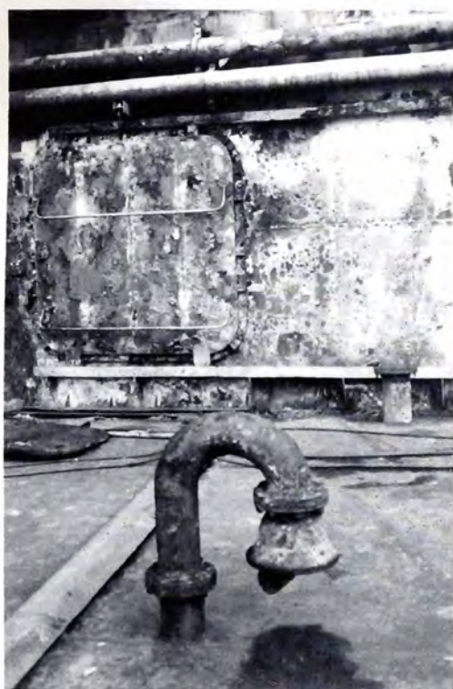
Damage to Omi Yukon's fuel-oil storage tank vent, located port-side forward.
