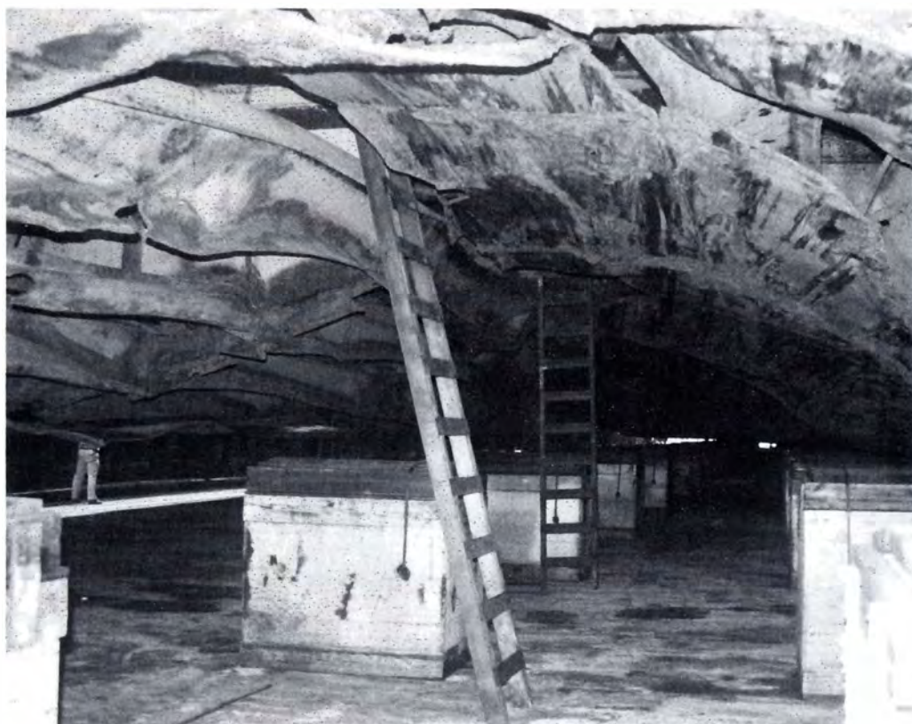
Raking damage inflicted on the hull of Exxon Valdez.
