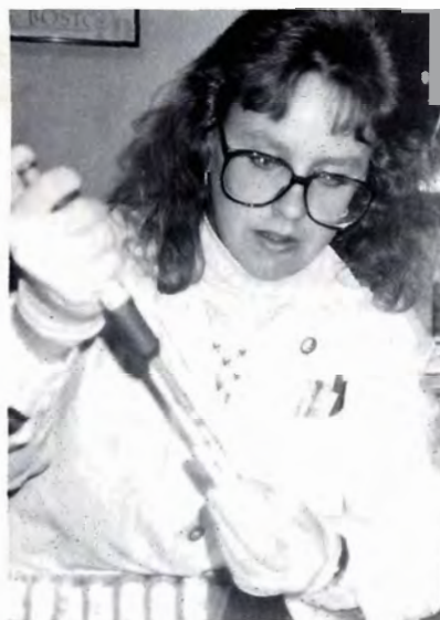
Step 6) (left) Chemicals are mixed into a "positive" aliquot to prepare for a "confirmation" test. Step 7) (below) Centrifugal force machine separates drug properties from the aliquot, forming a concentrate.
