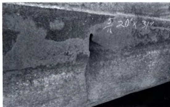
(below) The hull of the Apex 2002 was torn away from a wing-void bulkhead by the explosion.
