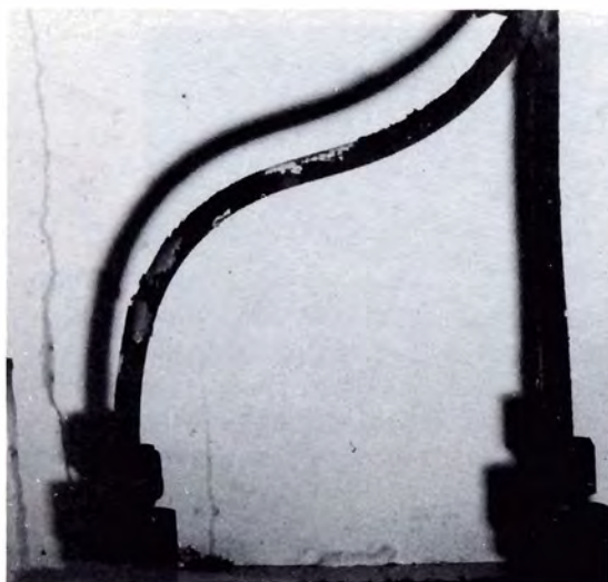
The blackened condition of brass and copper sewage treatment unit components indicate the presence of hydrogen sulfide.
