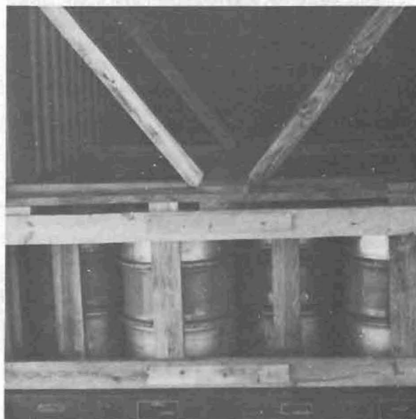
Excellent securing of methyl isocyanate. (Photo courtesy of the author)
