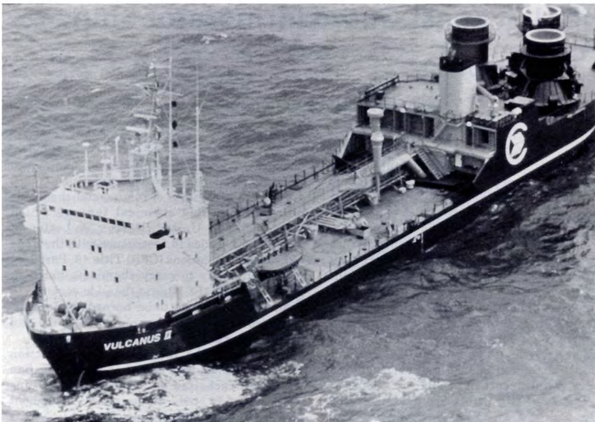
The foreign-flag vessel Vulcanus II was the first vessel to be certified by the Coast Guard as an incinerator ship under Public Law 97-389. (Photo courtesy of Chemical Waste Management, Inc.)
