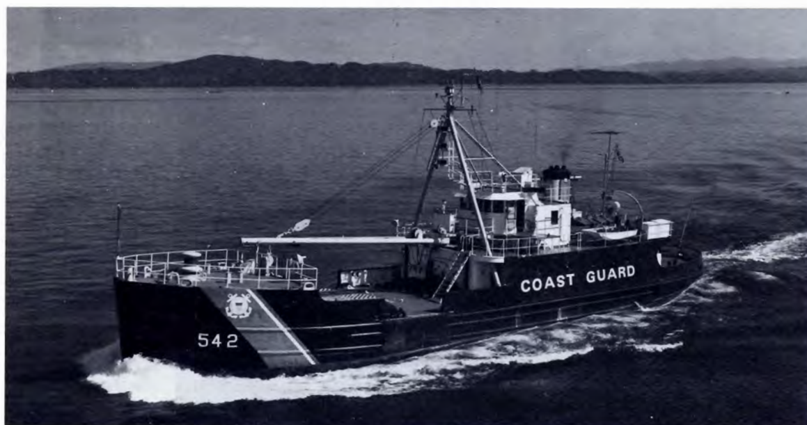
This coastal buoy tender maintains aids to navigation in coastal waters, performs SAR and law enforcement missions, and participates in special assignments.
