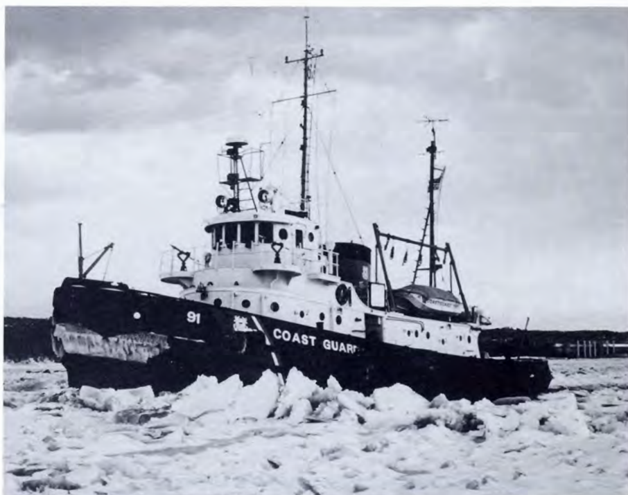
This 110-foot tug is used for breaking ice and for coastal search and rescue missions.
