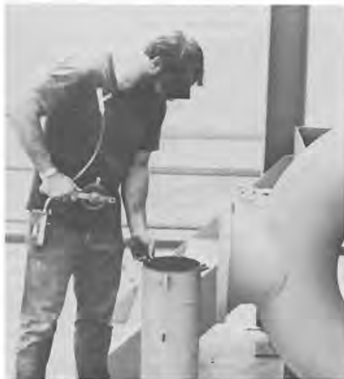
This employee is using a restricted gauging device. Since the sounding tape extends to the liquid in the tank, there is little danger of his breathing dangerous vapors. Note the non-standard apparel; originality in a dress code is not recommended.
