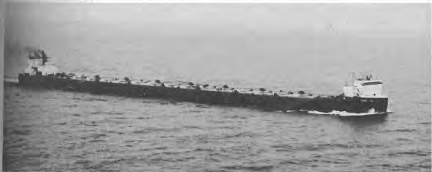
The unusually large length-to-beam ratio of Great Lakes ore carriers like the M/V STEWART J. CORT makes them subject to significant springing vibratory stresses.
