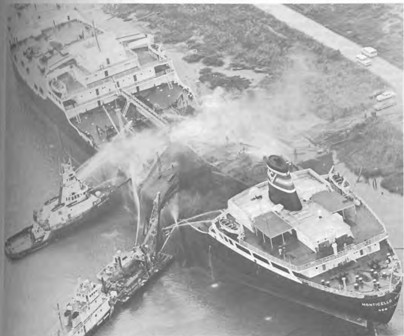
The internal tank explosion literally peeled open the main deck of the MONTICELLO VICTORY.
