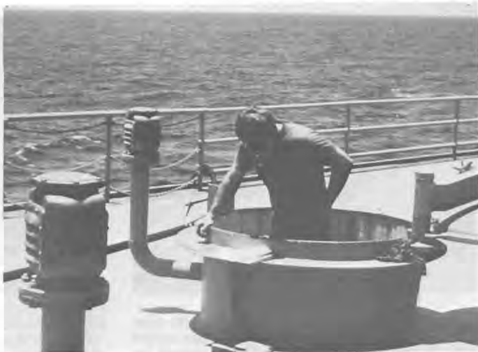
"Gee, I'm brave." Here we have a man entering a tank with poor skin protection, no respiratory protection, and no support team on deck.
