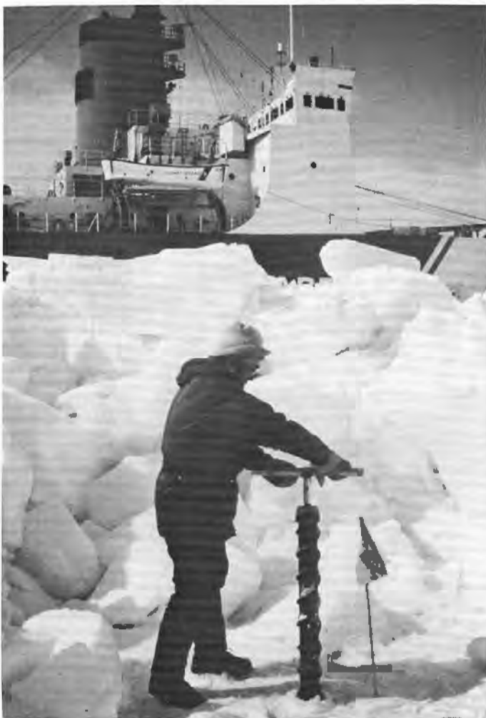
A scientist takes ice samples during MarAd's trafficability tests. In the background is one of the Coast Guard's polar-class icebreakers.
