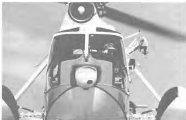
The FLIR is enclosed in a turret on the nose of the aircraft.
