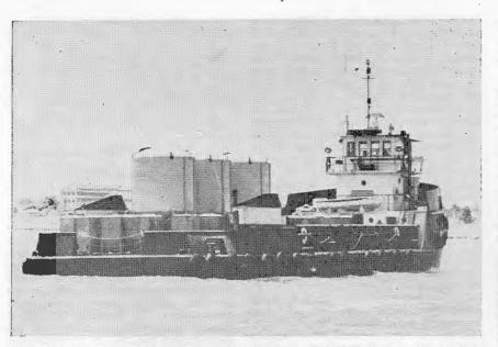
ONE EXAMPLE of an offshore supply vessel carrying heavy weights high above the waterline.
