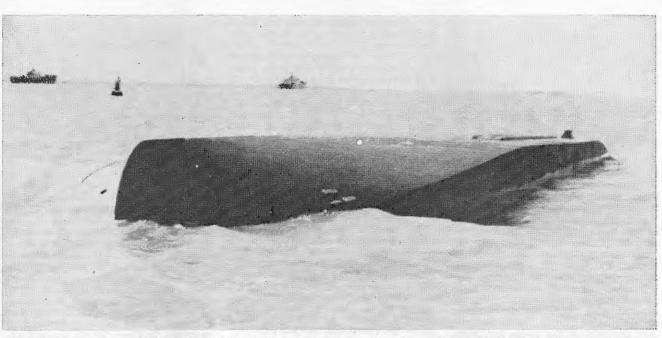
THE ABOVE picture shows what happens when the stability of a flat bottomed supply vessel is impaired by overloading or improper cargo stowage.
