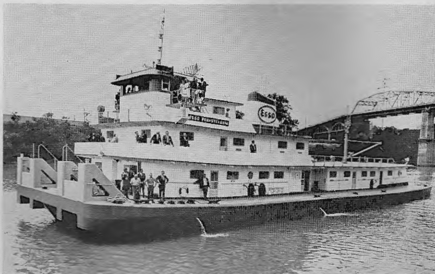
THE TOWBOAT Esso Pennsylvania shown underway shortly after her completion last year. Part of the fast growing inland-waterways fleet, the vessel, when pushing an eight-barge integrated tow, transports 17,000 to 180,000 barrel oil cargoes between Baton Rouge and Pittsburgh.
