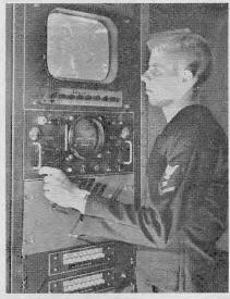
A TECHNICIAN adjusts controls on the transmitter of the Coast Guard's experimental television radar station at Sandy Hook, N.J. A picture of harbor activity from Ambrose Lightship to the Narrows is obtained from a high definition radar that scans the area.
