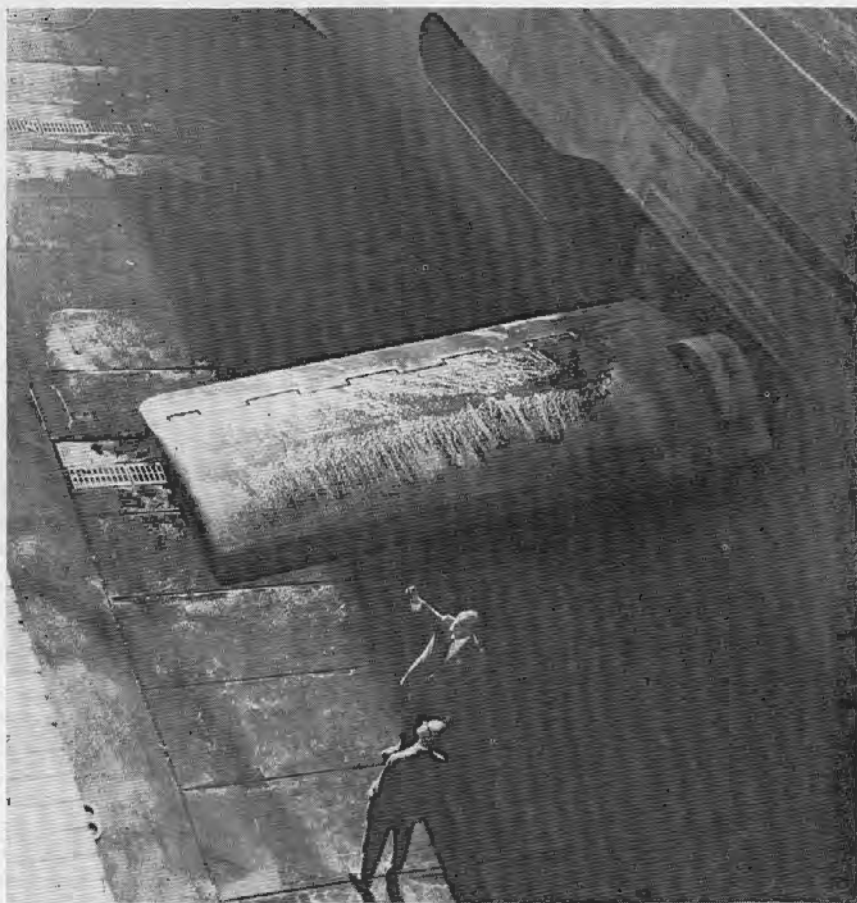
THE FINS are located amidships, some 18 feet below the surface of the water. Each winglike fin extends 14 feet from either side of the hull with the maneuverable flap at its after edge. Photo courtesy Sperry Gyroscope Co.
