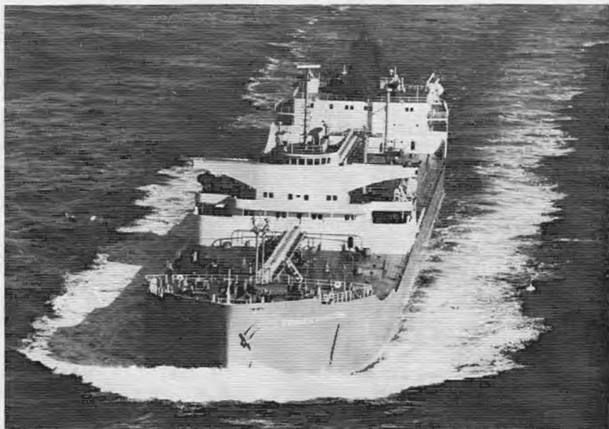
THE NEW 50,000 deadweight ton supertanker SS Pennsylvania Sun , biggest ship of the Sun Oil Co. fleet, plows ahead at 17½ knots in the picture above. The 745-foot long ship, with a capacity of 417,000 barrels of oil, boasts the first 360-degree pilot house installed on a tanker. She is also equipped with a single channel ship-to-ship radiotelephone, two radar stations, true motion radar repeater, dead reckoning analyzer, and a stern anchor.
