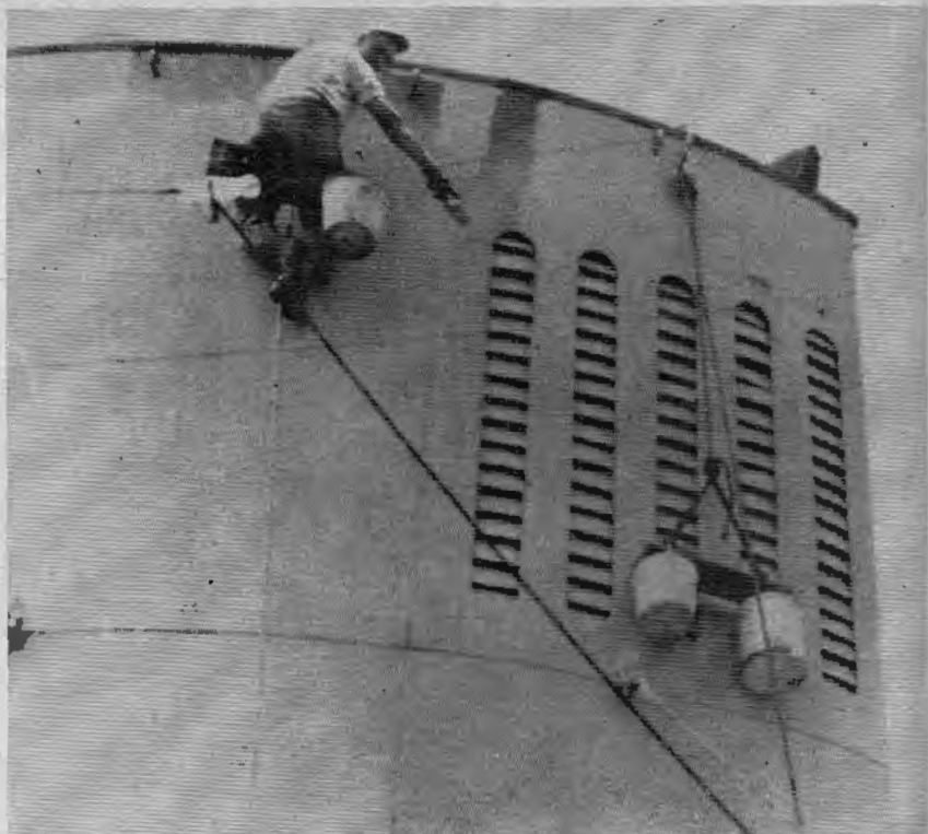
HIGH ATOP THIS SHIP'S stack a seaman points out the position a fellow crewmember was in when his gantline parted plummeting him to the deck 25 feet below.
