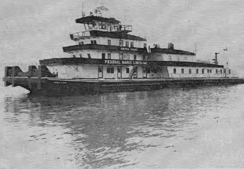
LARGEST AND MOST POWERFUL inland towboat is the MV United States seen above. With 8,500 horsepower, she is capable of pushing 40 barges carrying a total of 40,000 tons of cargo—equivalent to the capacity of 10 freight trains of 100 cars each. The towboat is 180-feet in length, has a 58-foot beam, and displaces 1,760 tons at an operating draft of 8 feet 6 inches. Photo Courtesy Federal Barge Lines, Inc.
