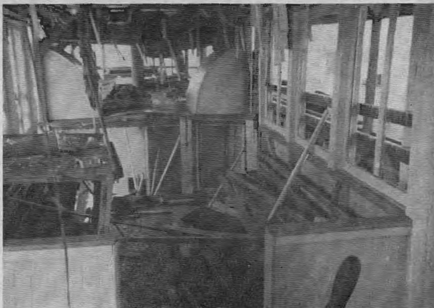
INTERIOR VIEW of a 53-foot passenger motorboat taken after an explosion of a 10-pound CO 2 portable extinguisher. There were no casualties in this case.
