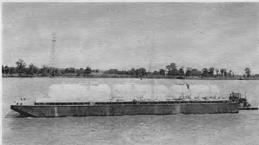
A COMMON SIGHT on the inland waterways is the propane or anhydrous ammonia barge seen above. Carried "piggy-back" in a typical hopper type barge they permit the use of smaller barges with more economical drafts. Photo Courtesy St. Louis Shipbuilding and Steel Co.
