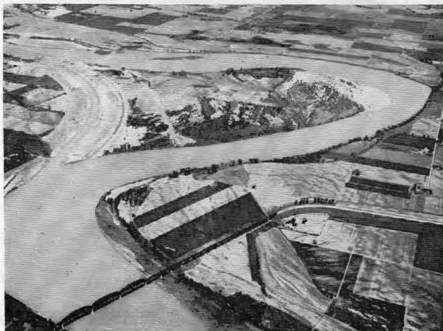
A NAVIGATIONAL improvement is seen in this aerial photograph on the Missouri River. The pilot canal, 1.7 miles long, has eliminated this long bend in the river and shortened the route approximately 2.6 miles. Note the land beginning to accrete in the old channel. Photo Courtesy Corps of Engineers.
