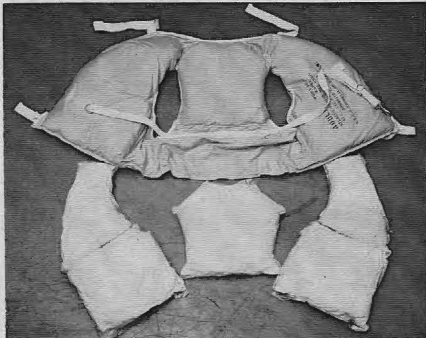
COAST GUARD APPROVED life preservers manufactured since September 24, 1958, must have the kapok or fibrous glass filler fitted in a plastic envelope. The top part of this photograph illustrates a complete Model 3 life preserver, and the bottom part shows the plastic encased pads prior to insertion. Previously approved life preservers may be placed in service and/or continued in service as long as in good and serviceable condition.
