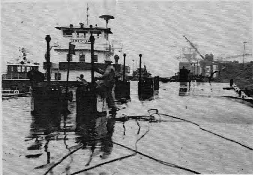
CLAD IN SOU-WESTER and oil skins, a Coast Guard inspector prepares to enter a tank barge to determine the cause of the swelling seen in this picture.
