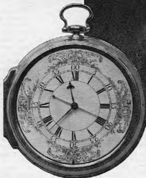
Chronometer No. 4, completed 1769. Actually a large watch, it was instrument which actually won the Board of Longitude's prize.
