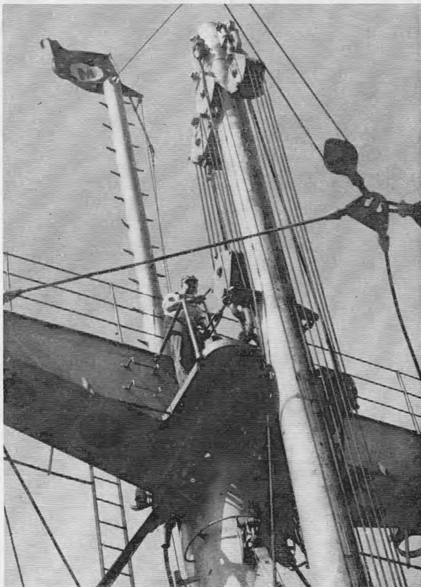
Figure 1. Seaman shown aloft preparing to let go turnbuckles securing 30-ton boom on Victory type vessel. Note number of parts at moving block.
