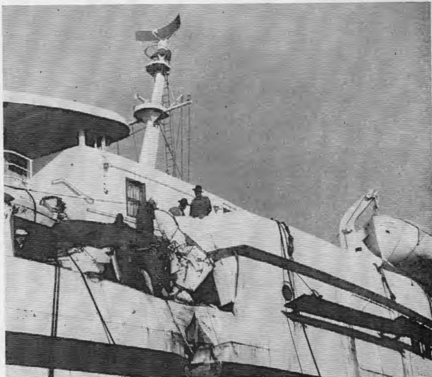
RADAR EQUIPPED: Port side view of the MV Chinook after collision in the Puget Sound. Note radar mast and antenna with unobstructed sweep of the horizon.
