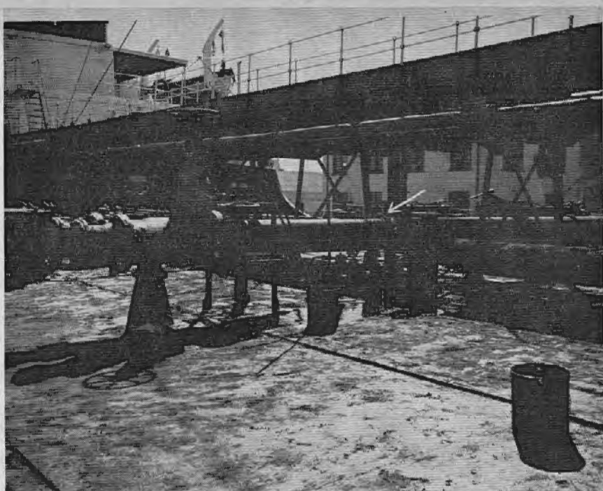
Figure 1.—Aft crossover line and coupling showing broken coupling forward of the line.
