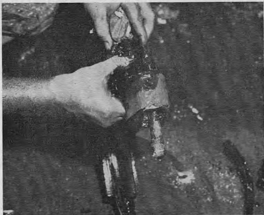
Figure 2.—Top housing of coupling showing wasted head of starboard bolt.
