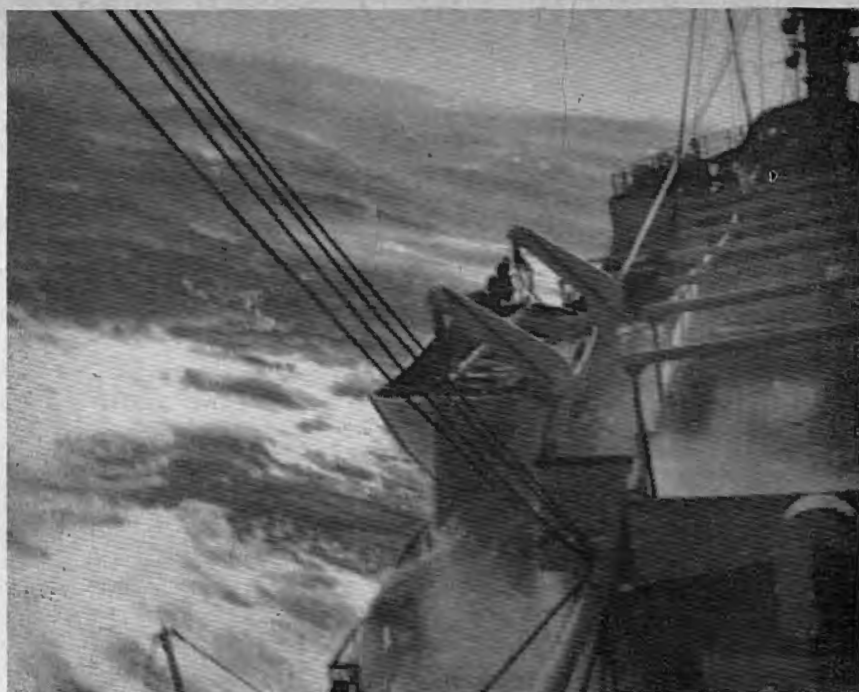
Figure 1. Riding out typhoon Ruth with stopped engines. Typhoon Ruth was the most violent storm the author ever experienced, but his ship came through undamaged by riding out the storm instead of fighting it.
