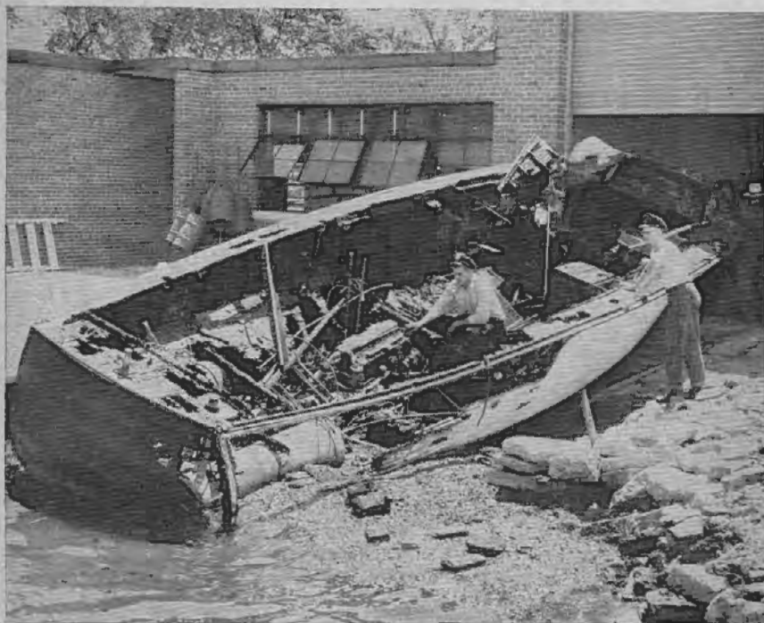
Figure 10. A leaking fuel line caused this fire.
