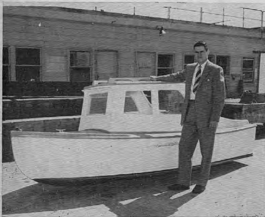
Figure 1 illustrates why this motorboat was topheavy. The man standing alongside is the Coast Guard Investigating Officer.
