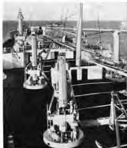
Very few cargo ships are equipped with such highly efficient means of cargo handling as individual cranes over each hold as in the view above of a foreign freighter.
