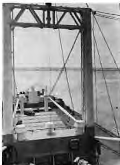
In common practice, the topping line from boom end runs to the top of the king post and is secured somewhere in the working area as shown in this typical deck view.
