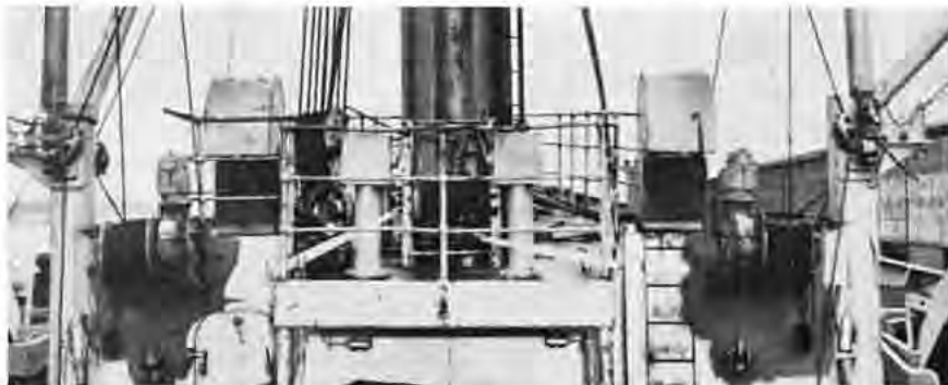
Here two American boom topping winches are mounted on a deck house completely removed from the main deck working area.
