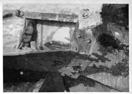
Starboard side looking forward at edge of curled-up deck plating. The cleavage fracture turns to shear in the vicinity of riveted seam and then back to cleavage beyond the seam.
