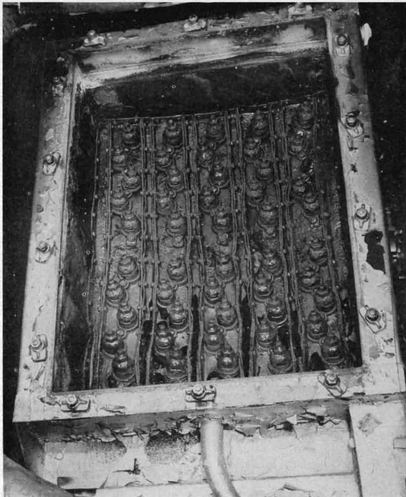
Boiler damaged by a soot fire. See page 106 for article on soot fires.
