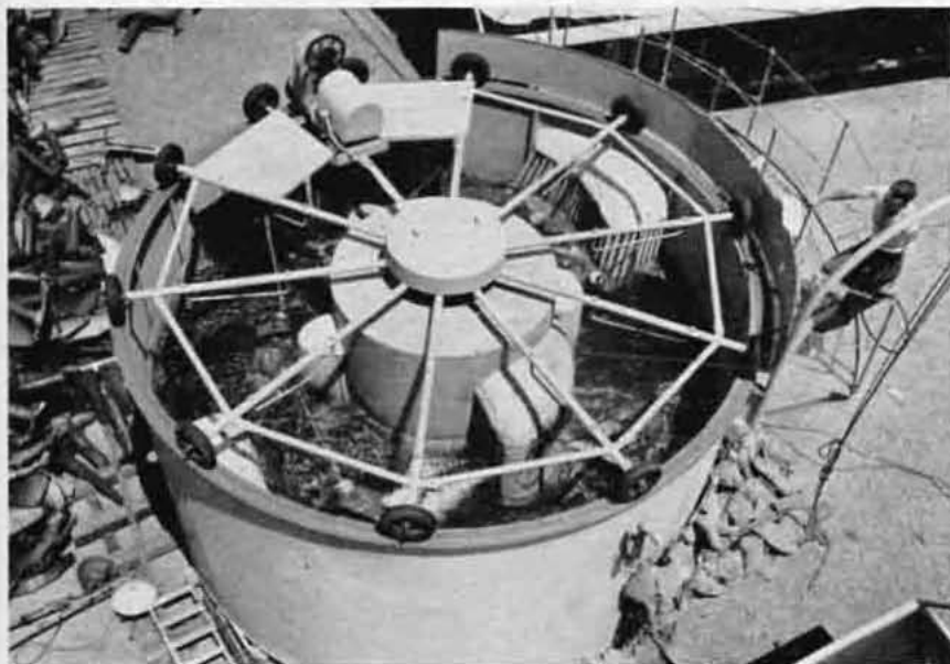
Life-jacket testing machine.
