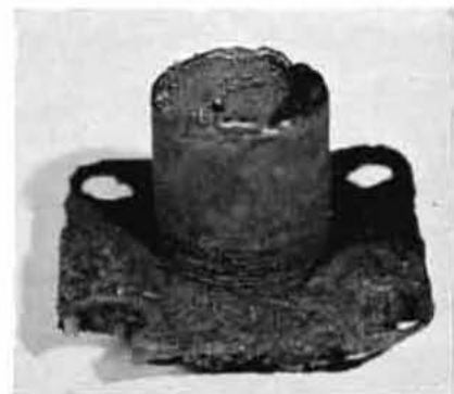
Internal flange connection with section of desuperheater line showing general corrosion and deterioration of threaded connection.
