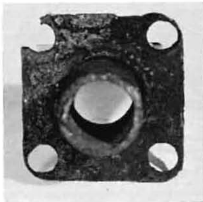
Internal flange fitting, desuperheater line, showing general corrosion and deterioration at threaded attachment.
